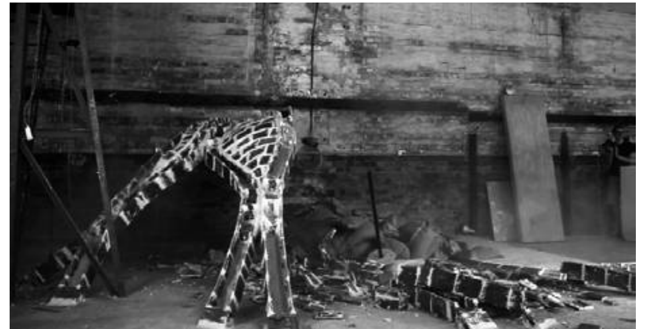
Figure 13. The Ribbed Catalan vault was subsequently tested, with no evidence of movement or failure at a point load of more than 1.5 tons. One of the ribs was then demolished in order to destabilise the structural integrity of the vault, after which the point load caused the failure of the vault. Photos: James Lauman.
