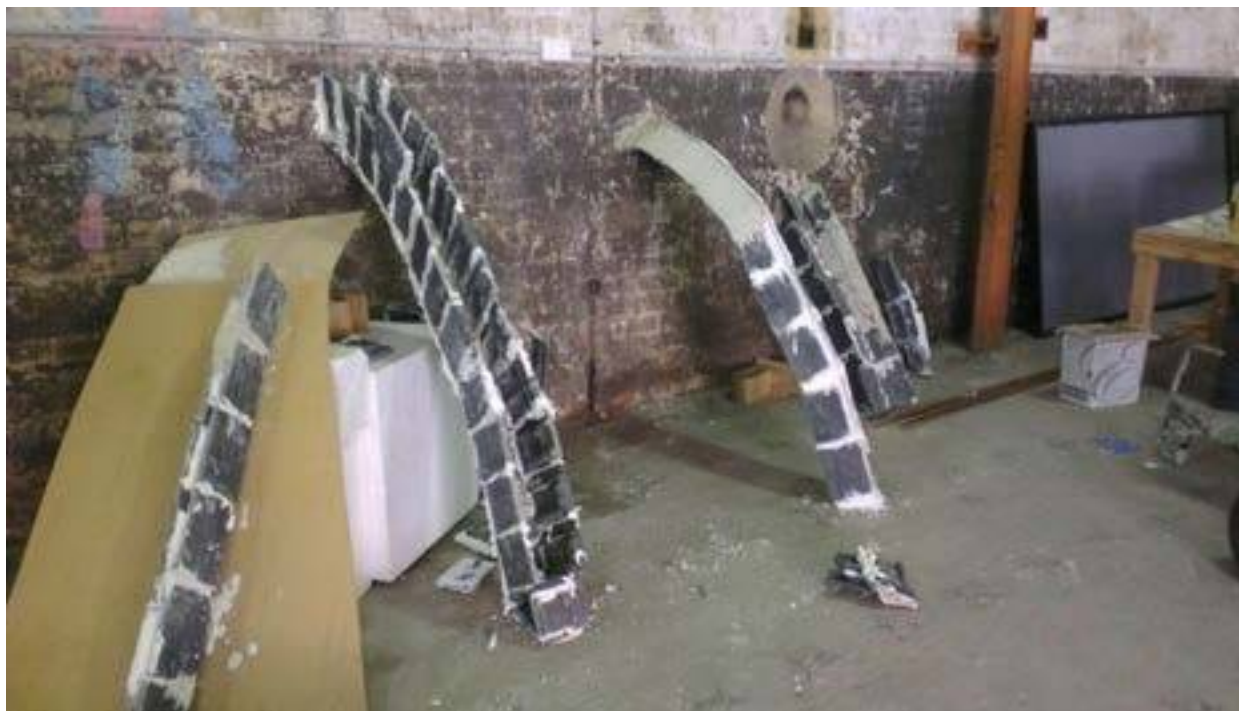
Figure 3. Initial prototypes produced to understand capacity and opportunities of ribbing with the available concrete tiles, Ribbed Catalan Masterclass, UTS, 2012. Photo: Melonie Bayl-Smith.
