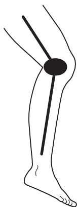
Fig. F4.3. A long-arm goniometer showing the alignment of the two measurement arms along the axes of the limbs and the central protractor
